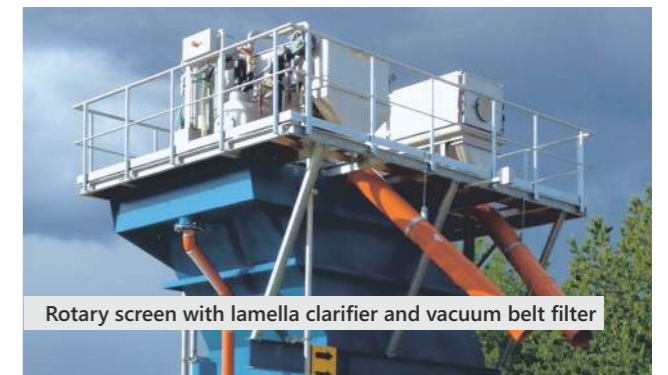
Rinsing water treatment airport catering
