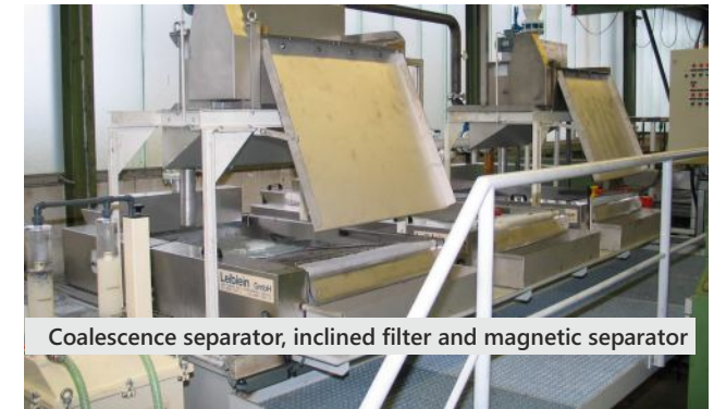
Central system with inclined filter and coalescence separator
